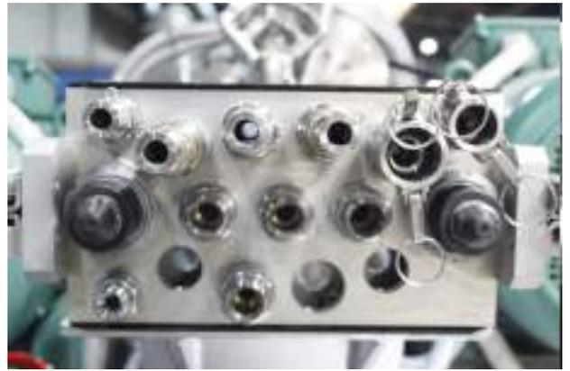
The linking pipes that connect the multi-connector and the machine are achieved with TRICOCLAIR pipes.
