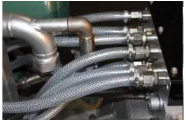
The four cooling water pipes are connected to a collector at the rear of the machine chassis.
