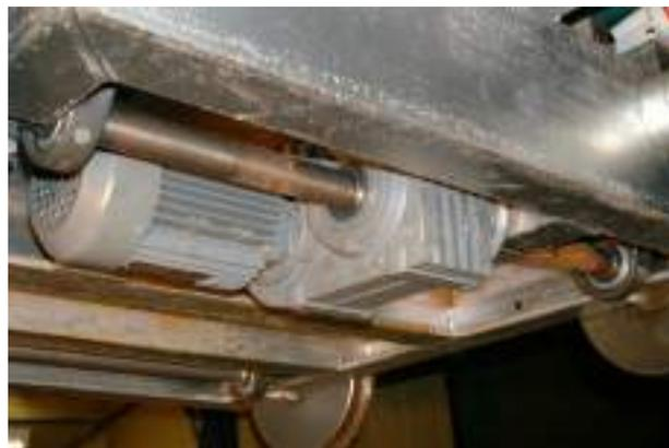
The longitudinal motion of the machine on the rails is ensured by a gear motor directly mounted on the rear shaft.
