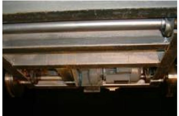
The machine suspension is ensured by anti-vibration mounts positioned between the bearings of the wheels and the chassis.
