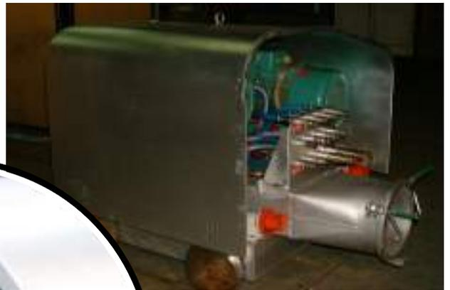
A safety guardrail is installed under the housing, at the rear of the machine. This system enables the access to the connectors but bars the access to the moving organs. This barrier can be removed when the housing is open.
