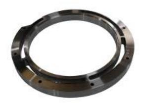
The stretching lips of spindles n°1 and 2 are held by an external flange which is screwed to the heart. The stretching lips of spindles n°4 and 3 are mounted separately. The stretching lips are wearing parts, thus they are screwed on the heart in order to make the replacement easier.
