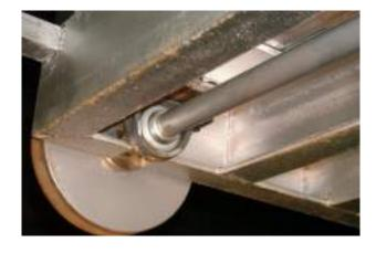
The machine suspension is ensured by anti-vibration mounts positioned between the bearings of the wheels and the chassis.
