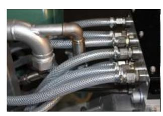
The four cooling water pipes are connected to a collector at the rear of the machine chassis.
